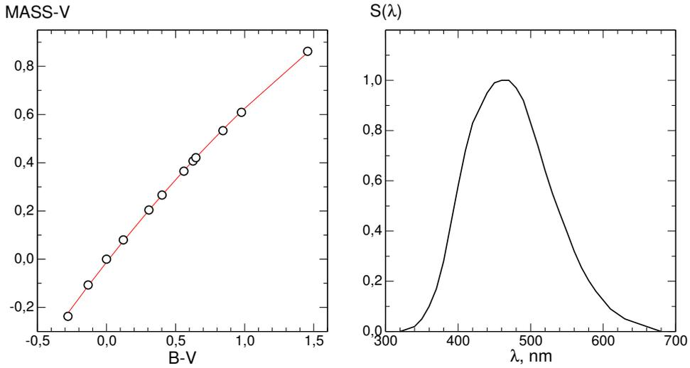
Figure 1.7: On left: Color equation between MASS magnitude and star color index B-V. On right: Spectral response of the ELT MASS device.
