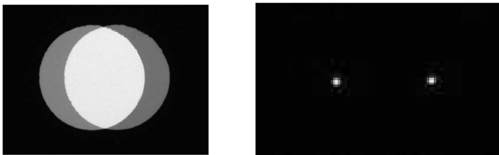
Figure 3.2: On left: The CCD frame of the illuminated field aperture. On right: Right aligned artificial star images with the horizontal separation of 41 pixels.
