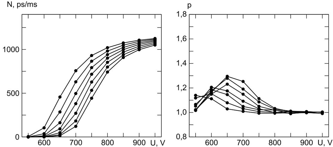
Figure 4.2: Light counting functions. Left: Flux dependence on the high voltage for 7 threshold levels (0.3, 0.4, 0.5, 0.6, 0.7, 0.8 and 0.9 mV), lowest curve corresponds to the 0.9 mV level. Right: Non-Poisson parameter as a function of Voltage for 7 threshold levels, here lowest curve corresponds to the 0.3 mV threshold.
