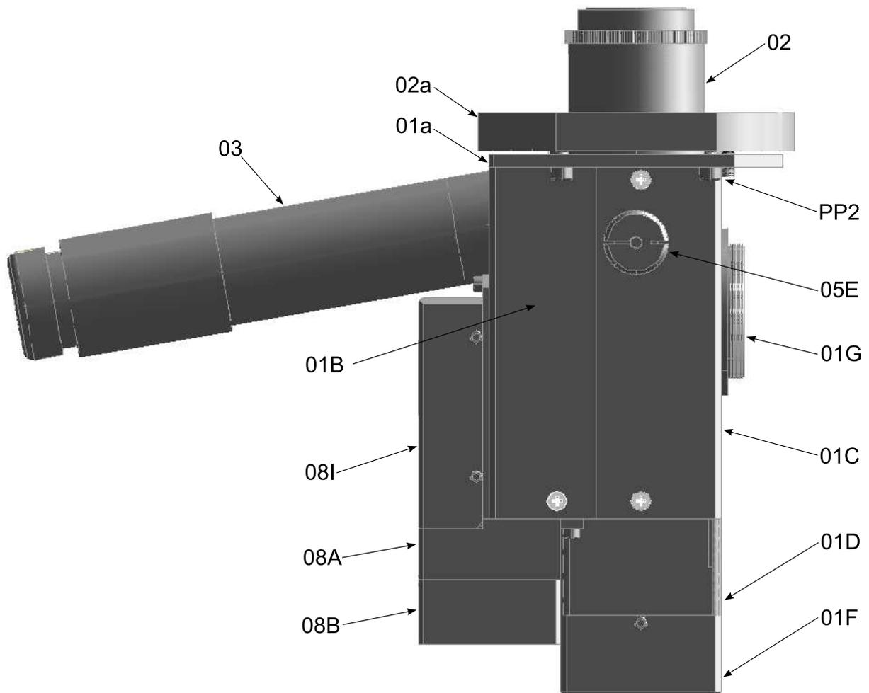
Figure 2.1: Side view of the MASS/DIMM device without CCD camera. See designations in text.
