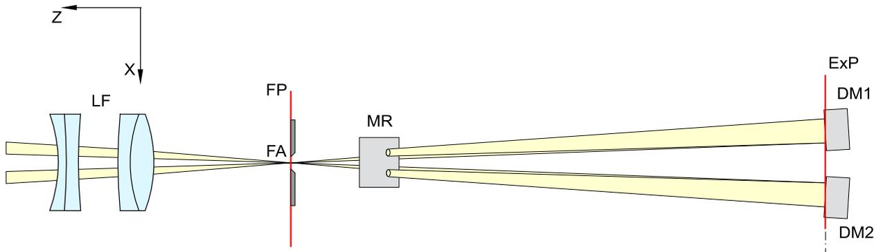
Figure 1.8: Optical layout of DIMM sub-device in ZX plane (corresponds to the top view in Fig 1.4). The MASS sub-device and viewer are not shown. Common part: LF — Fabry lens, FP — instrument focal plane, FA — field aperture, ExP — plane of exit pupil and mask. DIMM: DM1 and DM2 — DIMM re-imaging mirrors, MR — folding mirror.
