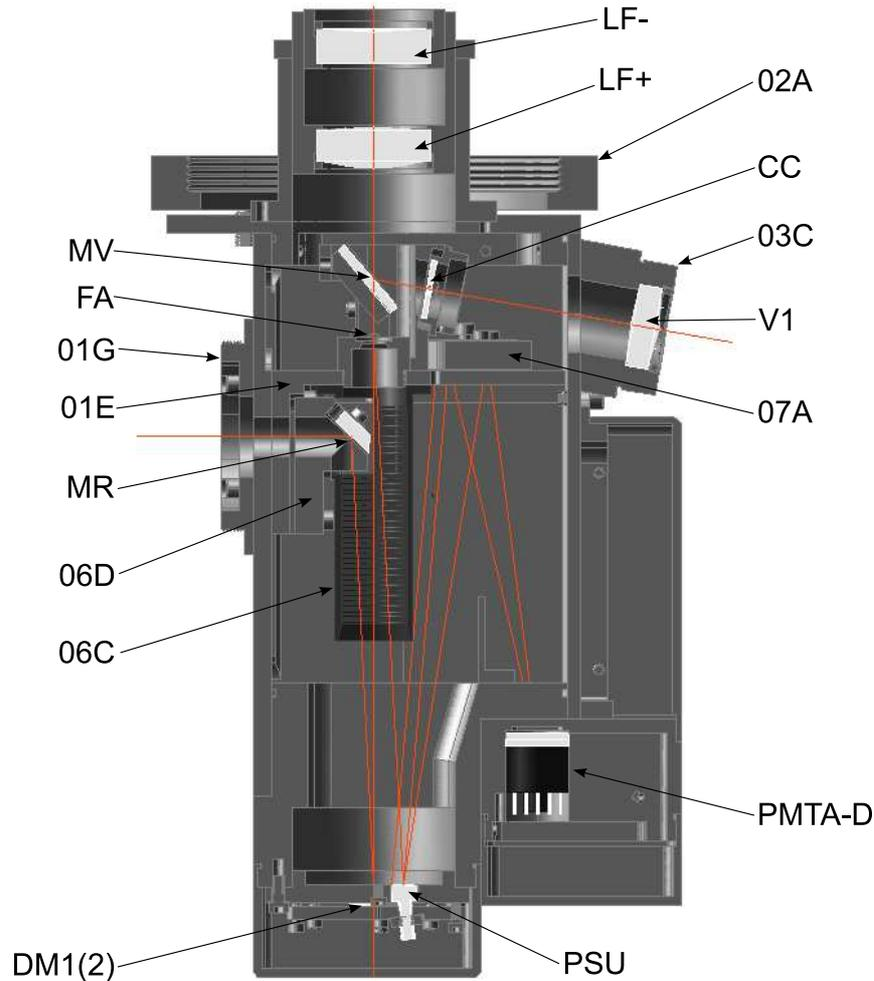
Figure 2.2: Cross-section view of the MASS/DIMM device.
