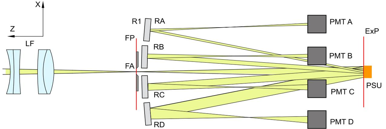
Figure 1.5: Optical layout of the MASS sub-device in ZX plane (corresponds to the bottom view in Fig 1.4). DIMM sub-device and viewer are not shown. Common part: LF — Fabry lens, FP — instrument focal plane, FA — field aperture, ExP — plane of exit pupil. MASS: PSU — pupil segmentation unit, RA, RB, RC, RD — re-imaging mirrors of the A-, B-, C-, and D-channels, PMT — four detectors.
