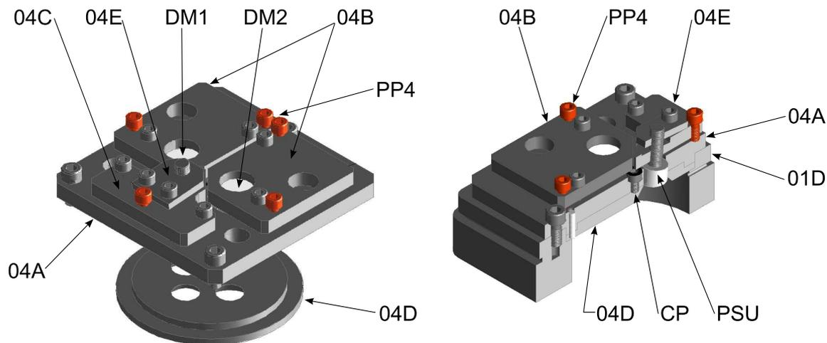
Figure 2.5: The view of the optical plate with PSU holder and two DIMM mirrors alignment plane.
