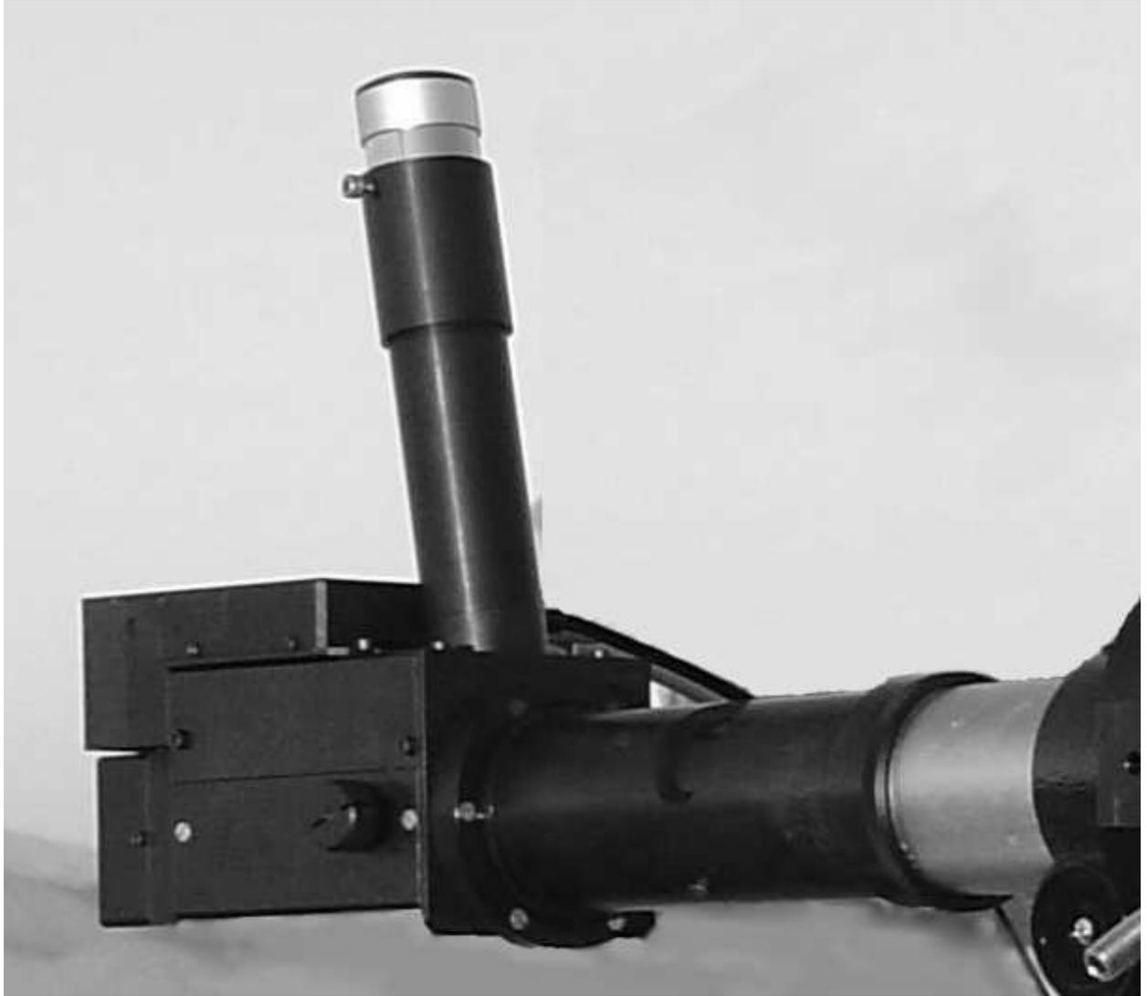
Figure 2.1: MASS device attached to refractor, which is installed atop of the La Silla DIMM.
