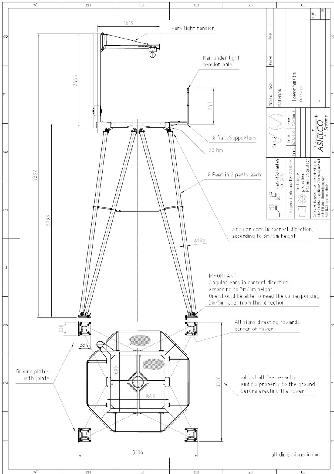
**Figure 5:** the ASTELCO tower requires minimum foundations of 4 concrete blocks, each 40cm x 40cm, 60cm deep, with a leveling accuracy of  $\pm 5$ mm over a distance of 2m. The total weight, with the enclosure is 1.4 tons. The tower can be assembled by 3 persons with one car, one tackle, ropes and small tools.
