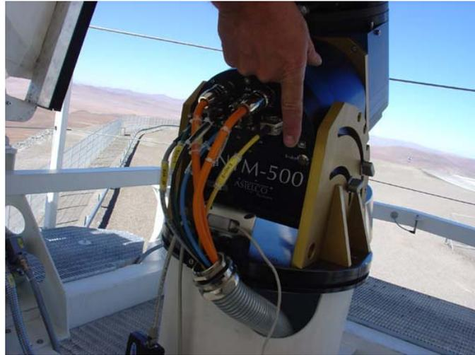
**Figure 7: releasing the pneumatic brake (on both axes simultaneously)**
