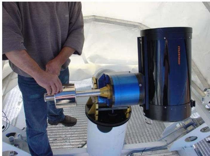
**Figure 9: balancing the mount in RA**
