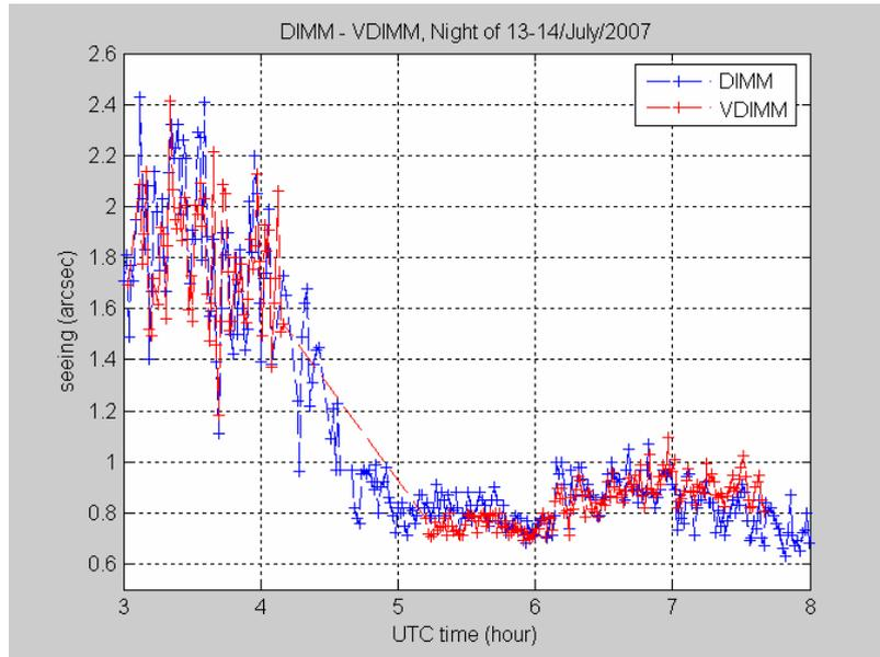
Figure 16: The Turbina DIMM (at 2m above ground, red) was compared at Paranal to the ESO DIMM (at 6m, blue) in July 2007.
