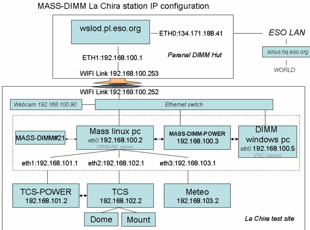
**Figure 11: La Chira Station IP configuration (note that MASS-DIMM instrument is powered from the mount 12V auxiliary power supply)**
