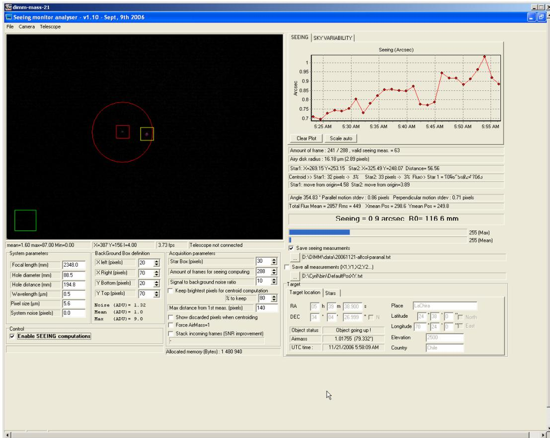
**Figure 17: The DIMM software used for the preliminary operation is a window based shareware developed by Cyril Cavadore. The detector is a Phillips SPC900NC ToUCam III webcam set at 5ms exposure time. The frame rate was 8.5Hz with real time determination of the centroids.**
