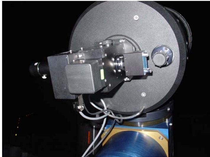
**Figure 13:** the camera is installed such as the X axis is parallel to the pupil segmentators separation (here vertical)
