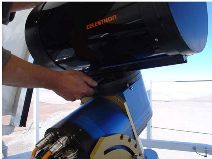
**Figure 8: sliding the optics along the dovetail to balance the mount in DEC**
