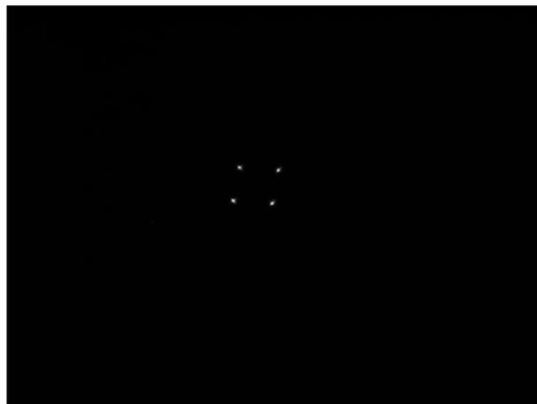
**Figure 14:** MD#21 plate scale calibration on the double star HD2884/2885 (Bet Tuc, 00 31 32.5, -62 57 29) of separation 26.6": the pixel size is 0.66".
