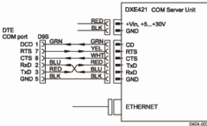
Disconnect the 3 wires TxD, RxD and GND from the DTE COM port (the connector is fixed to the opened door).
