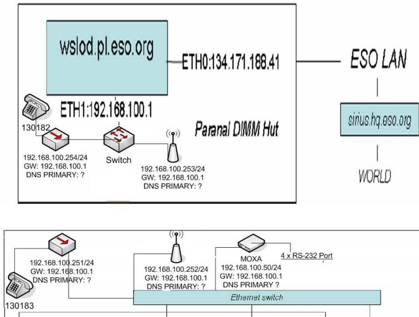
Figure 12: Paranal-La Chira wireless link configuration
